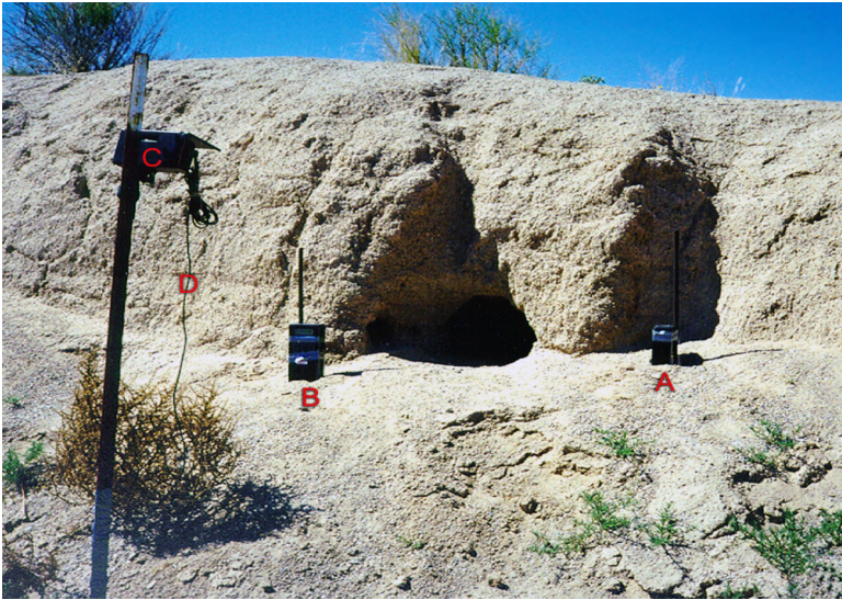
Figure 1. TrailMaster (TM1500) camera system set up at a burrow (A, transmitter; B, receiver; C, camera and protective shelter; D, cable).
